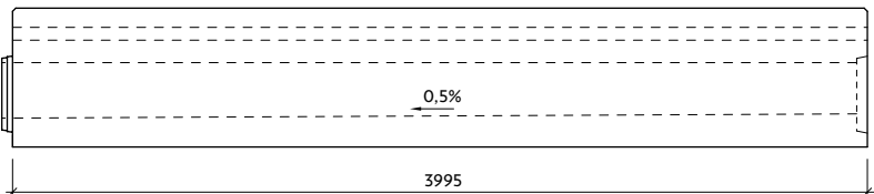
Profile I-6-G24/26-L 0.5% flow profile bottom gradient
