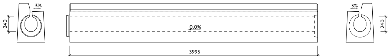
Profile I-3-T24/24-L - without internal flow gradient
