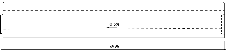
Profile I-6-G22/24-L 0.5% flow profile bottom gradient
