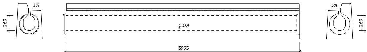
Profile I-3-T26/26-L - without internal flow gradient
